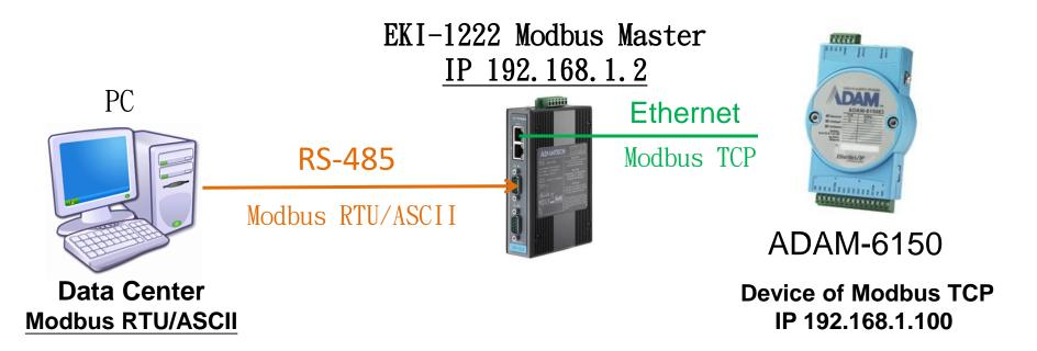
The behavior of Modbus gateway which translates the data format of Modbus from RTU/ASCII to TCP, that we calls "Master Mode"
